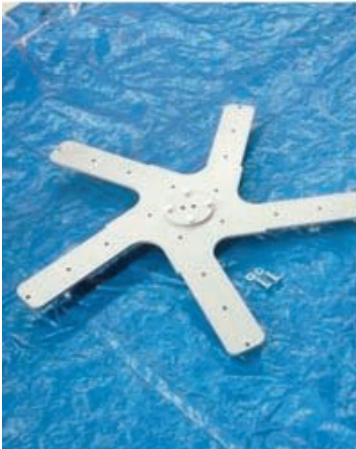
AFTER DISASSEMBLED BLADE SUPPORT, DISASSEMBLY HUB
